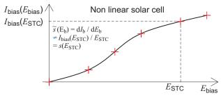
Fig. 7 Short-circuit current of non-linear solar cell with bias irradiation.
