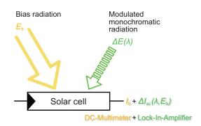
Fig. 8 Dual-beam optical arrangement.
