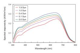
Fig. 5 Non-linearity of spectral responsivity of DSC.
