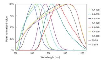
Fig. 13 Spectral responsivity of reference cells.
