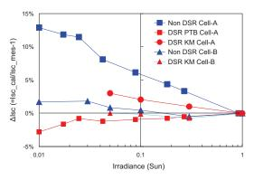
Fig. 17 ΔI<sub>sc</sub> comparison between DSR and Non-DSR methods
