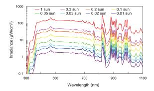
Fig. 16 Spectral irradiance of solar simulator A.
