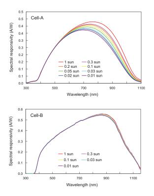
Fig. 15 Spectral responsivity of non-linear device under various irradiances.
