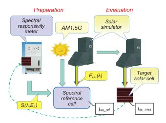
Fig. 6 Measuring principle structure of spectral reference cell.
