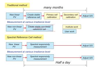
Fig. 4 Solar simulator adjustment process: Traditional method vs. Spectral Reference Cell method.
