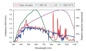
Fig. 3 Irradiance distribution of solar simulator and AM1.5G and relative spectral responsivity of c-Si cell and DSC.
