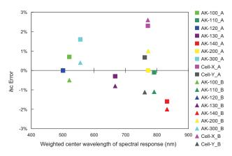
Fig. 14  $\Delta I_{sc}$  for various spectral responsivities of linear cells with solar simulators A and B.
