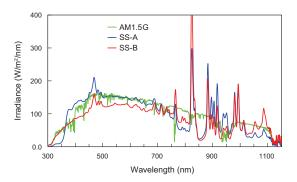
Fig. 11 Irradiance of solar simulator.
